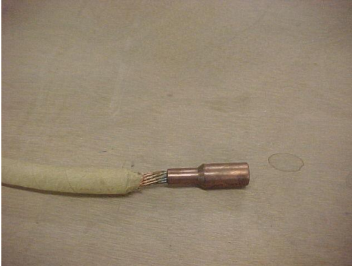
Figure 9 Cable stripped of insulation and inserted into crimp connector.
