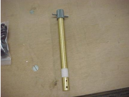
Figure 6 Shaft (cotter pin taped to shaft)
