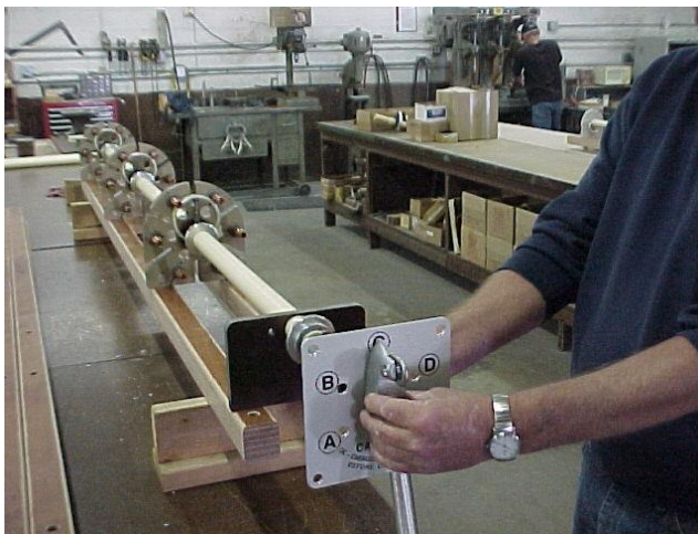
Figure 17 Switch in NOMINAL position, handle in NOMINAL position according to Index plate (position C or 3 on a 5- position switch).
