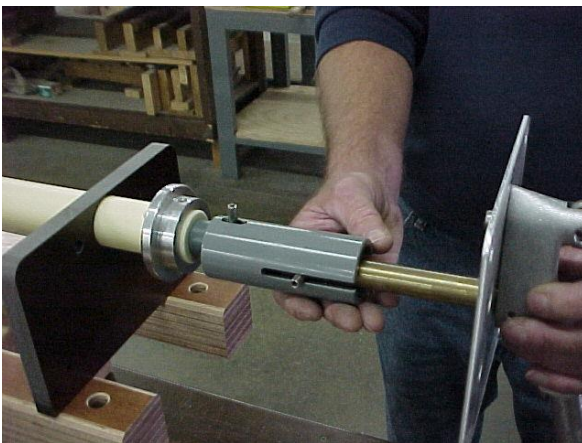
Figure 16 Pins located approximately center of slot.
