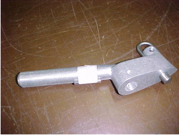
Figure 19 Handle with external spring pin taped to it.
