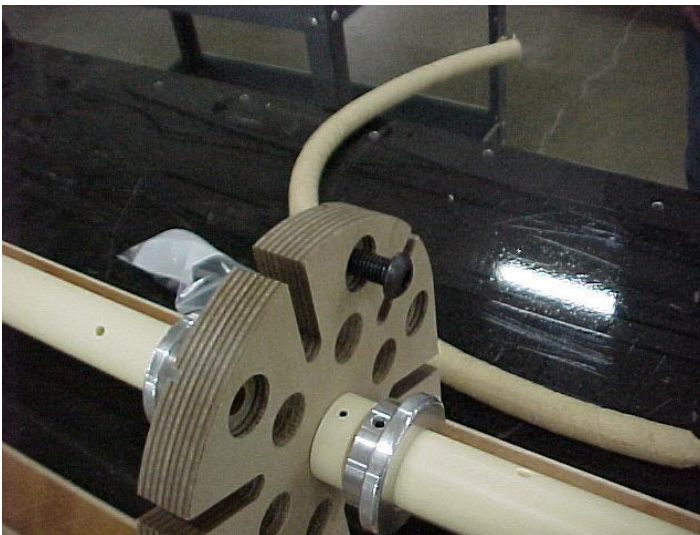
Figure 10 Hex Head Cap Screw being inserted into a non-molded deck.
