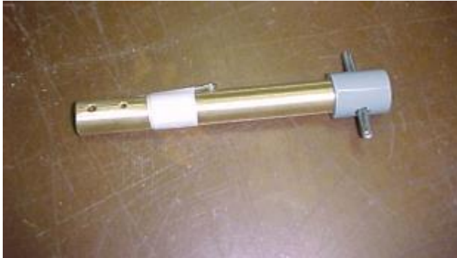
Figure 18 Shaft w/cotter pin taped
