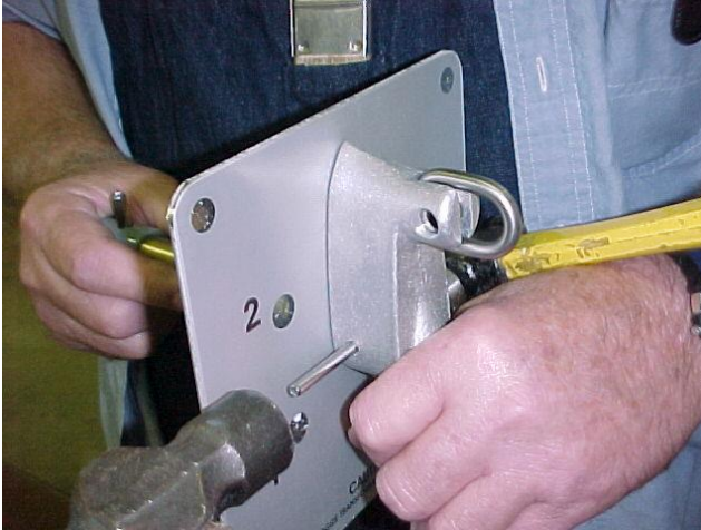
Figure 22 Support must be provided as spring pin is inserted into shaft. In this picture a hammer is used on right side of handle to support the shaft as pin is driven in with hammer from left side of handle.
